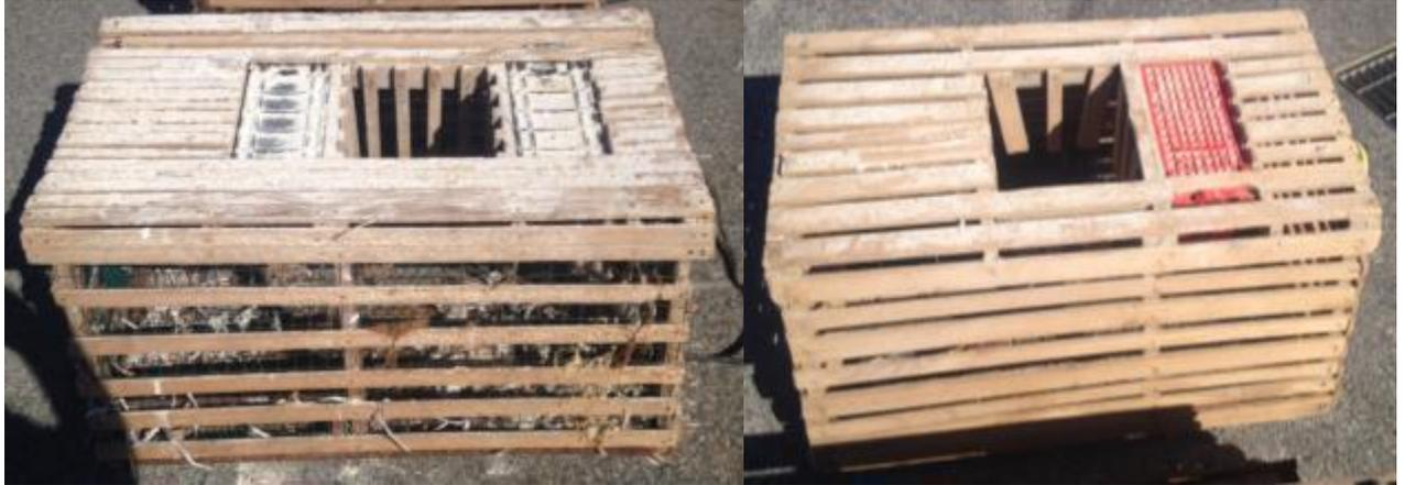
Figure 3 Image of two types of meshed pots with plastic coated wire mesh (left) and extra battens (right)
